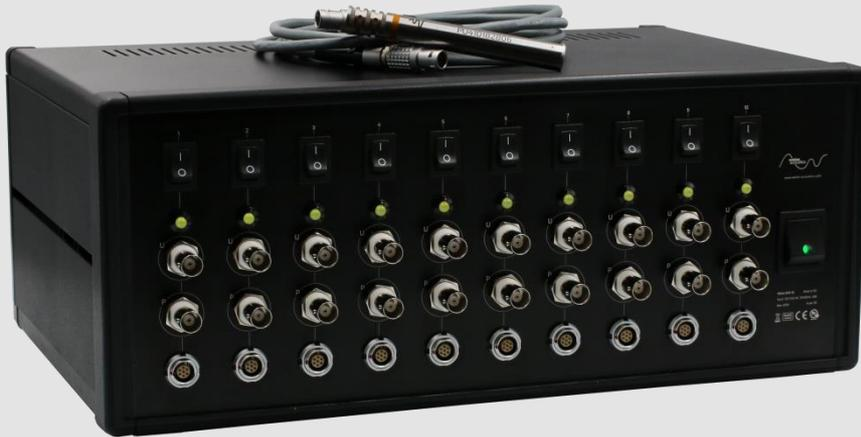
Weles Acoustics' Weles BOX X is a modular device designed to support up to 10 standard WA101 1/2" PU Sound Probes. Each probe can be operated separately through a dedicated Weles BOX card equipped with its own individual power switch, probe input port and 2 analog BNC output channels - First channel for sound pressure, second for particle velocity.
